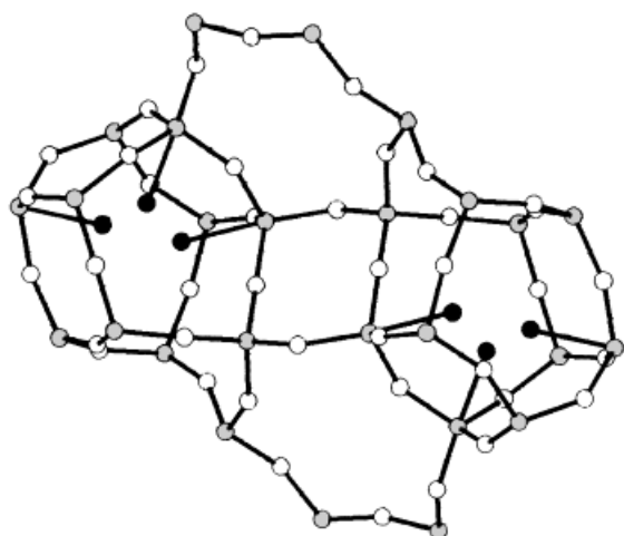
Figure 1. Two of the characteristic subunits of SSZ-23 (see text for further details). The diagram also shows the location of the partially occupied fluorine sites inside the small cages. Si atoms are shown as grey spheres, O atoms as clear spheres, and F atoms as black spheres.
